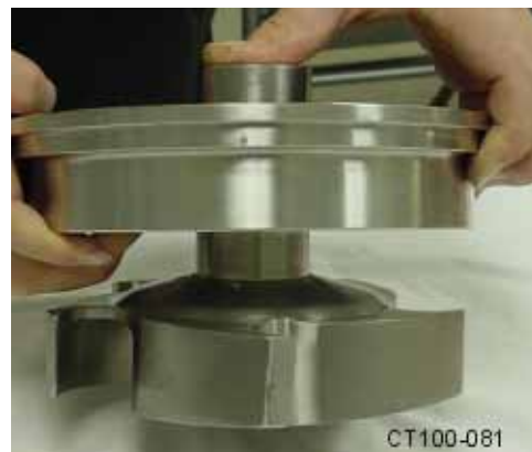
Figure 16 - Moving the Rotary Seal up the Shaft
