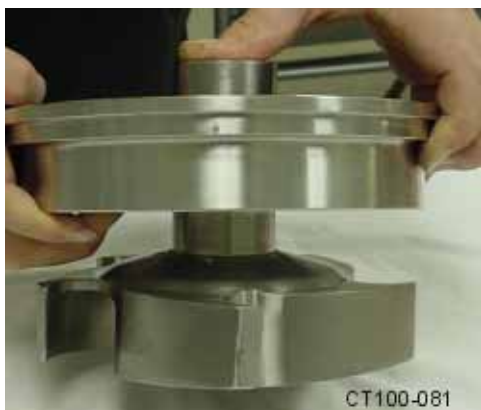
Figure 3 - Moving the Rotary Seal up the Shaft
